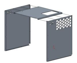
Once the side walls and top cover are loosely bolted together, install the back sheet into the cage. Hand tight only (leave all nuts loose).
